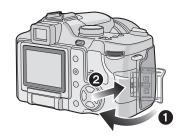
If the card door cannot be completely closed, remove the card and insert it again.
