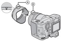
■ When removing the lens hood Press lock release button ⊚ and remove the lens hood.
